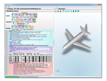
AVID ACS (AirCraft Synthesis) is a widely-used interdisciplinary aircraft synthesis program for application in the early design stages of an aircraft and can be used in conceptual design studies of numerous vehicles. From small UAVs to supersonic STOVL fighters, ACS is an excellent tool for getting the right answer earlier in the design process. ACS' computational speed means feedback for design changes is obtained in a matter of seconds.
