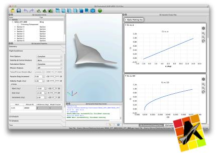
**AVID APEX** (Aerodynamic Prediction Express) is a comprehensive, medium-fidelity aerodynamic analysis tool designed to analyze full aircraft configurations. APEX is capable of analyzing complex geometries through the subsonic, transonic and supersonic flight regimes.
